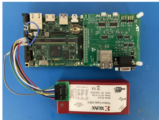
Figure 12: Enclustra ST3 with a Mars SoC Module and AIT PHY board
